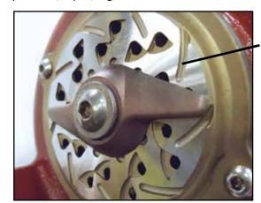
Exclusion cleanout slots and back relief clears debris from under cutter
