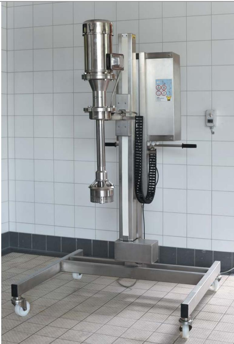
YTRON-Y Shear Jet, produce
