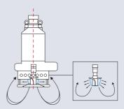
The rigid agitator delivers kinetic energy (energy of motion) to stir solids surrounding the pump intake, re-suspending them into a fluid state for easy pumping.
