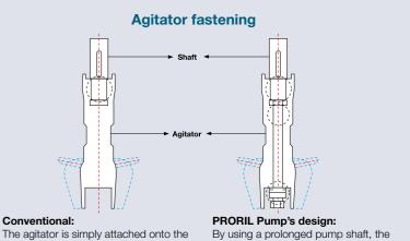
end of the pump shaft. As the agitator is only fastened at a single point, the agitator can loosen itself or come off during use.
