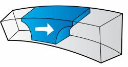
The deep channels in which the rotors travel provide large voids to minimize shear and bruising of solids.
