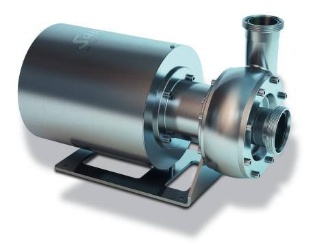
The flow optimised impeller and volute allow a very silent, gentle and efficient handling of the liquids. The dead space free and hygienic design guarantees fast cleaning and complete draining.
