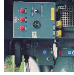
Auto-start control panel saves fuel and running hours.
