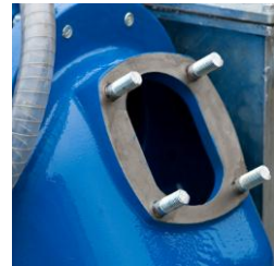
Inspection cover on volute
