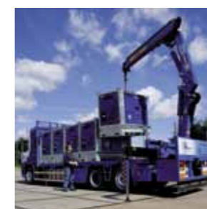
Easy to transport and store. Two compact pumps can be loaded crosswise on a truck, and even stacked.
