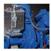
**Large inspection** covers Full access to suction line, float box, impeller and valve.
