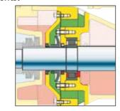
3 Pressure relief chamber Makes it impossible for any fluid to enter the bearing housing.
