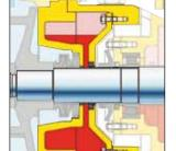
1 Large oil chamber For optimal cooling when running dry or in snore mode.
