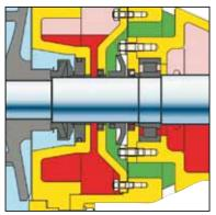
Oil chamber and pressure relief chamber
