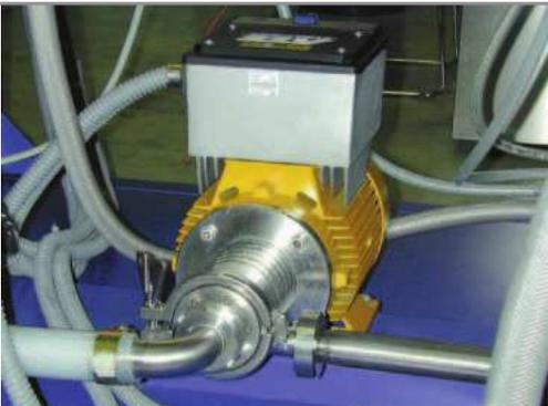
YTRON-Z with integrated frequency control
